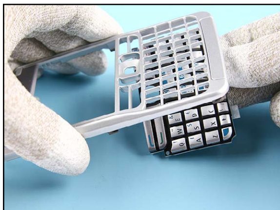
15. Separate the KEYMAT from the A-COVER ASSY.
