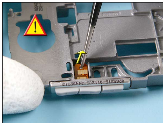
24. Unlock the SIDE BUTTON MODULE ASSY...
