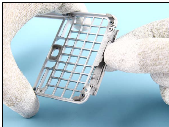
16. If needed, carefully unlock and remove the OPERATOR LOGO.
